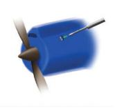
drill a hole in the cowl to match the position of the needle valve and insert a flat-blade screwdriver into the slot to adjust your motor.
