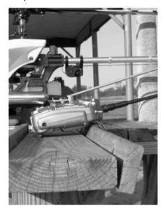
transmitter was sitting on the table, that rail would press up against the 'bind' button on the back. I would flip on the Tx switch, and then turn on the Rx, and
