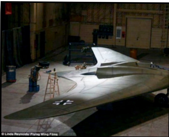
A full scale replica of the Ho 229 bomber made with materials available in the 1940s at preflight
