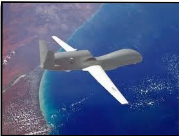
The Global Hawk flies along a pre-programmed flight path, but a pilot monitors the aircraft during its flight via a sensor suite which provides infra-red and visual images.
