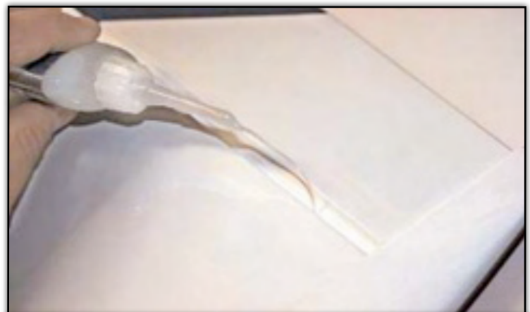
Once you have the control and fixed surface mated, remove the pins, flex the surface to the maximum desired deflection, and apply thin CA directly to the hinge as recommended.
