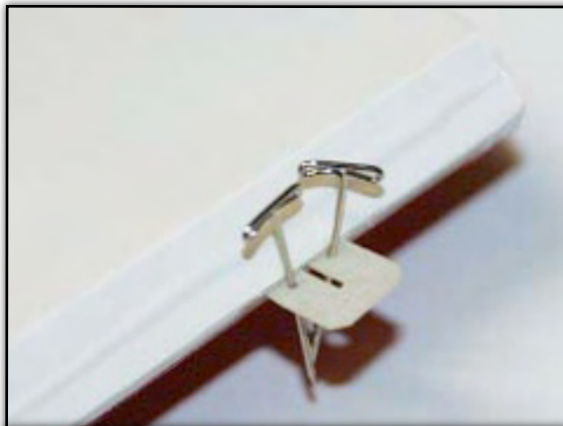
Two T-pins center a CA hinge in place during installing
