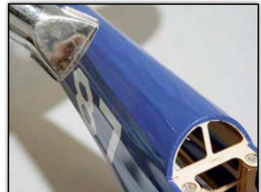
A heat gun can shrink the covering much faster than a covering iron, but you also run the risk of melting through your covering or having seams open up.
