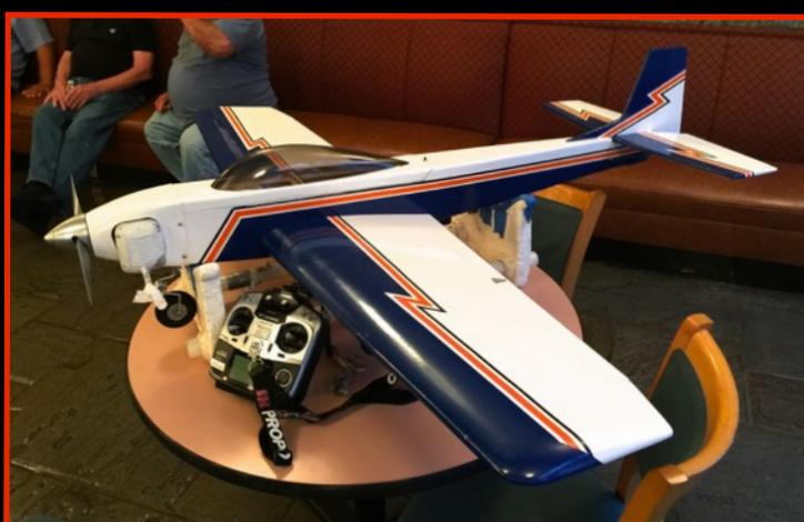
Nelson Ramos showed off his newly completed 60 size KAOS in which he went nuts on a whole lot of cool stuff including inverting the engine, using an inverted muffler instead of the standard one, an on board glow system and the use of a complete buss servo system.
