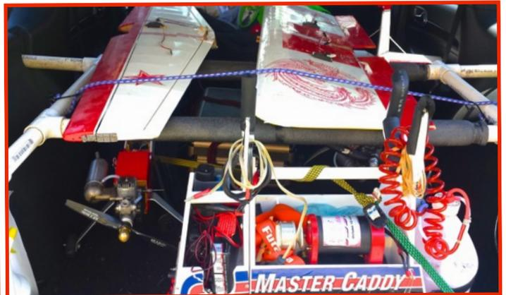
*"Dennis in these photos I tried to show how bungy cords are used to keep things like wings and tool box secure during transportation. I took this design from Nelson when I saw his Dodge station wagon he used to have. I used several "T" elbow and straight PVC pieces to fit my Jeep. I also used neoprene insulation tubes to protect the plane covering that has not been damaged yet by hanger rash. That's about all I can think of..."*
