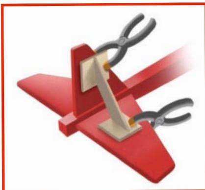
When I glued a vertical fin to an aircraft, I always had difficulty keeping it at 90 degrees to the stabilizer. Eventually I made a jig to solve this problem. First, I installed the stabilizer. After the glue had dried, I used my 90-degree jig to hold the fin in place. Just clamp it to the stabilizer and then to the fin. Keep everything clamped while the epoxy cures, and then unclamp the jig, and you'll find the vertical fin in perfect alignment.
