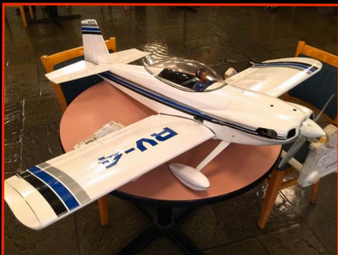
Curtis Underdue showed off his Great Planes RV-4 built from a kit which has a Thundertiger .77 4 Stroke. It's covered in monocoat. He started it in 2006 and finally finished it this year.
