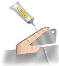
strengthen the area around the hole. If the wood ever splits, chances are the CA hinge material will hold.
