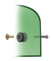
the fuselage with servo screws. The cowl now rides on the rubber grommets and is less likely to crack around the attachment holes. If you use JR's brass eyelets, you'll be able to attach your cowl with 4-40 bolts.
