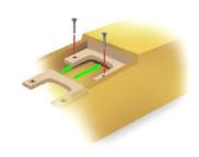
Then mark the spots where the wing bolts will come through the blind nuts into the balsa and drill them out. Shave out recesses for the blind nuts in the balsa backing block so that it can sit flat under the wing mount; then CA it into position. The blind nuts will never pop free again.
