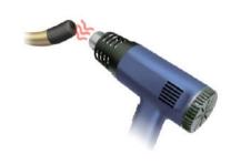
little hanging over the end to prevent the tube from cutting the fuel tubing. The shrink-wrap will seal so tightly to the brass tube that it won't leak after you shrink it.
