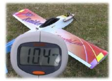
at something and pull the trigger. So long as you keep the trigger held down the speed is displayed in real-time. When you release the trigger only the highest speed recorded during that trigger-down period is displayed.
