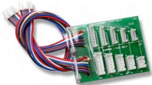
Above is the adapter board for a CellPro 10S for the Kokam JST XE (top) and Align JST XH (AL) (bottom) balance taps. Note that each connector size is only used once and has one more connection than cells in the battery.
