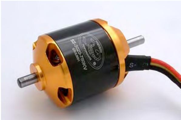
Scorpion has a motor that it calls the Scorpion SII-3020-780 weighing 166g. Scorpion uses the stator dimensions to designate its motor numbers. It has a Kv of 780 (about the same as the Hobby King motor). The C dimension is 37.5mm and B dimension is 45.7mm. The stator dimensions are 30mm x 20mm. Dimension A is 5mm. Scorpion does not give the useless maximum current but does rate this motor at a continuous 40 amps with a
