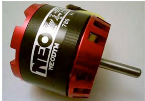
The Cermark NEO 25-780 has a similar 780Kv, but it only weighs 149g. Using its outside measurements it would be called a 42-40 780Kv. It has a 5mm shaft. It is rated for a maximum of 460 watts in and 55 amps. While it does use neodymium magnets, it would require a larger diameter prop with more pitch to achieve the same watts in as the other two motors. It is not similar to either of the other two motors, and its performance will be quite different.
