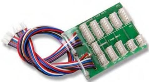
The photo of the second adapter board is for a CellPro 10S for the Thunder Power (TP) (bottom) and Polyquest (PQ) (top) balance taps. Polyquest uses the same connector for 2S, 3S and 4S packs and different connectors for 5S and 6S. Thunder Power uses the same connector for 2S and 3S packs and then a different one for 4S and 5S packs and double connector for 6S packs.
