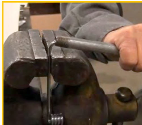
That's it. A simple and effective way to bend wire landing gear. Watch the video at https://www.youtube.com/watch?feature=player_embedded&v=6FZjfFW_7fE to see how easy it really is.
