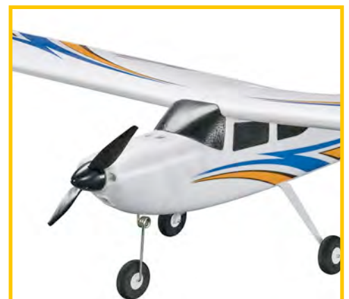
Above) your nose gear should be long enough so the model sits level or very slightly nose down for easy takeoffs and landings.
