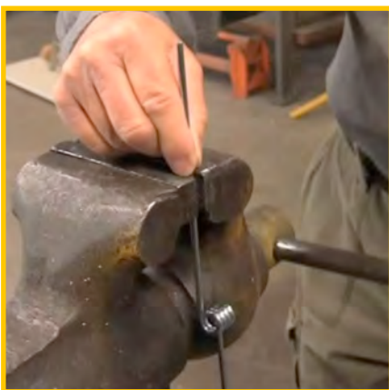
(Above) Here the wire gear has been clamped into a bench vise with the bend position at the top of the jaws.
