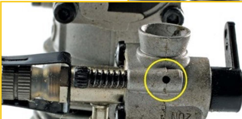
With a single-needle carb, there is a small air-bleed hole in the front for the low-end idle mixture. You adjust the mixture screw to open and close the hole to adjust
