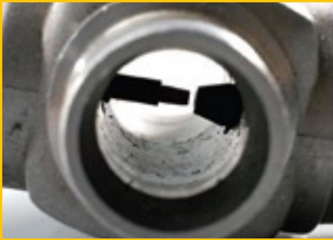
As the throttle barrel closes, the low-end needle assembly moves laterally into the fixed spray bar. This is why adjusting the low-end needle affects the high-end mixture adjustment.
