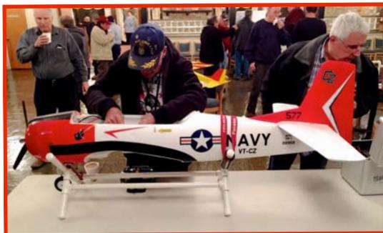
Jerry brought in the fuselage of an E-Flite CZ T-28 to demonstrate the sound board he installed. The sounds were of actual aircraft and the simul as ated sound of the radial engine in the T-28 increased in sound and rpmthe throttle was increased. Very Nice unit.
